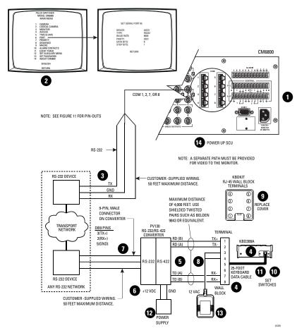
Figure 7. RS-232 Interface Connections (CM6800-48X8 Shown)
